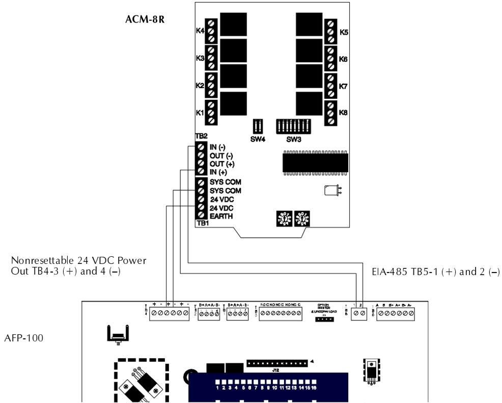
Figure 41 Wiring the ACM-8R
