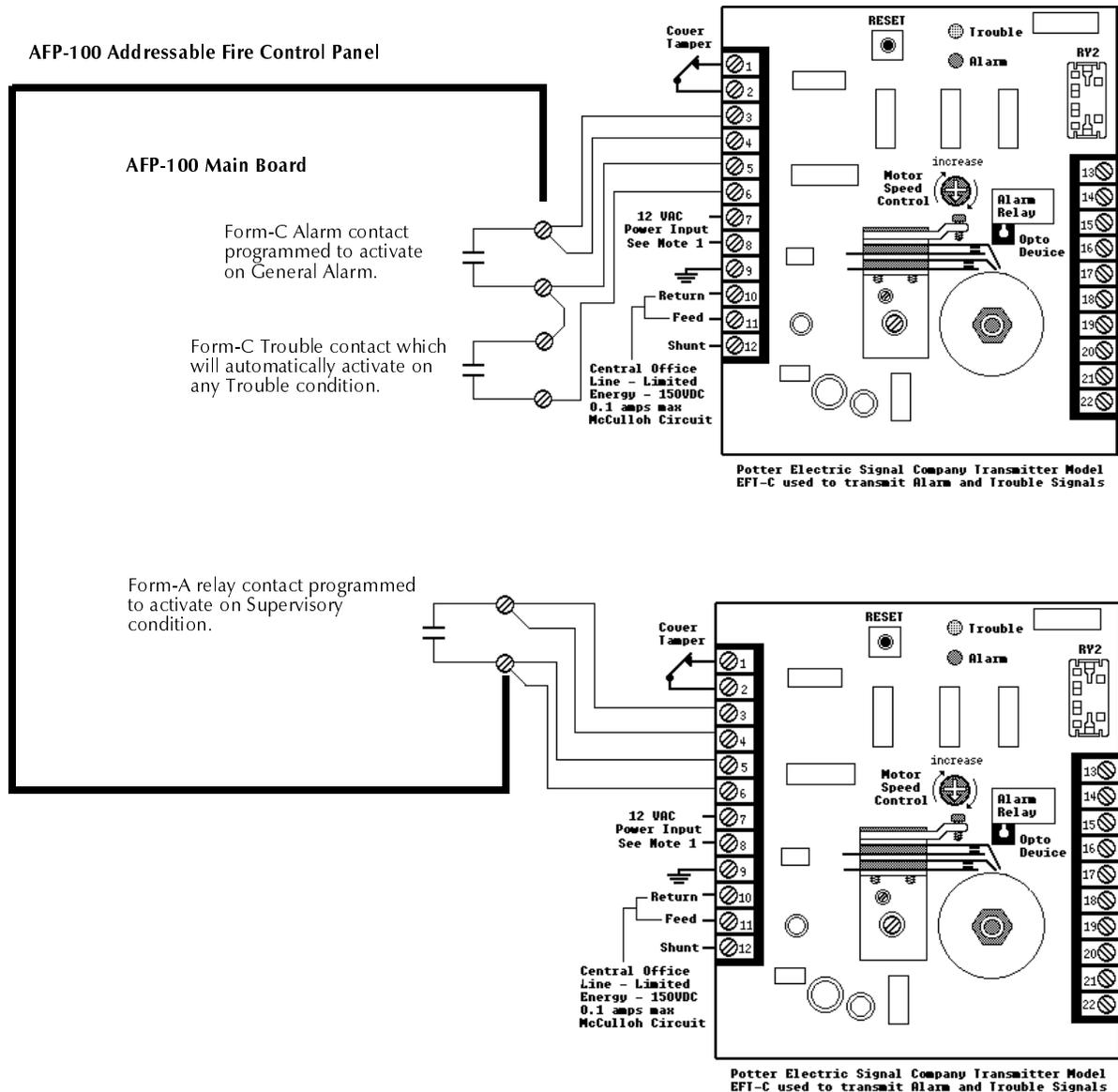
Figure 54 Proprietary Protective Signaling System
