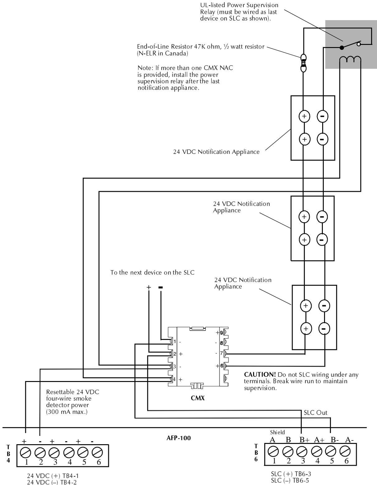
Figure 34 Style Y NAC using a CMX Module
