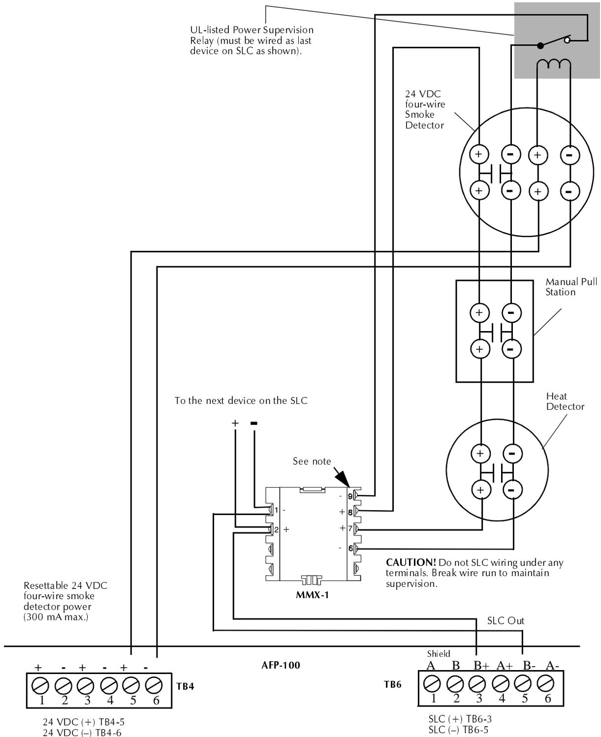
Figure 29 Style D IDC using an MMX-1 Module
