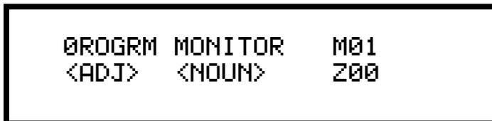
The major program editing for MMX modules is the selection of the Type Code on the first line. To change this selection, use the up and down arrow keys as the entire field blinks. The default selection is monitor as shown in the screen above. Note that selection of a Type Code may change the functional operation of the addressable device as shown in Table 9.
