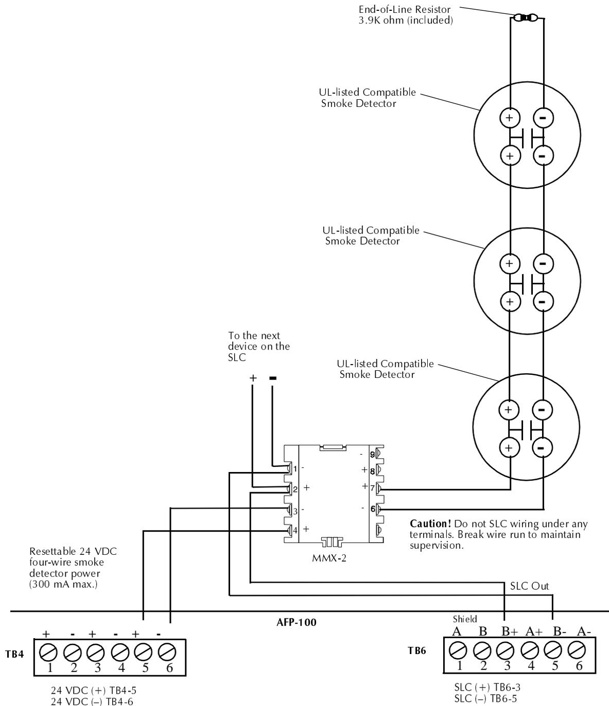
Figure 30 Style B IDC using an MMX-2 Module
