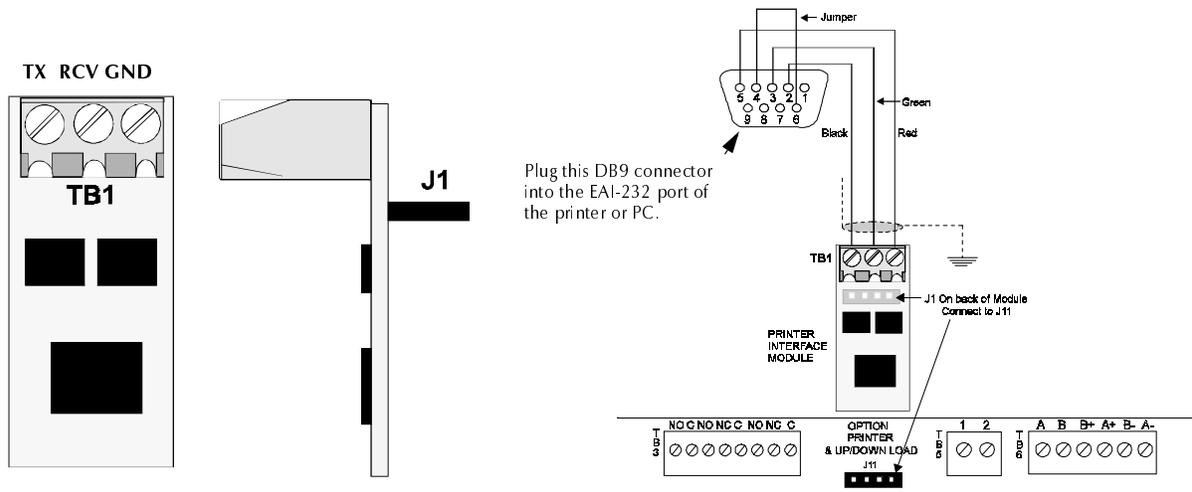
Figure 44 Remote Serial Printer and Computer Connections
