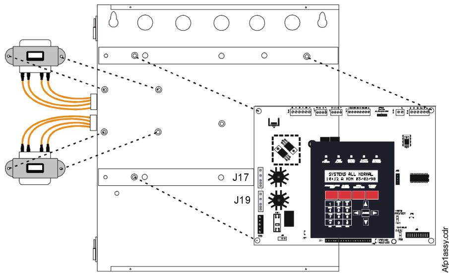
Figure 7 Component Mounting
