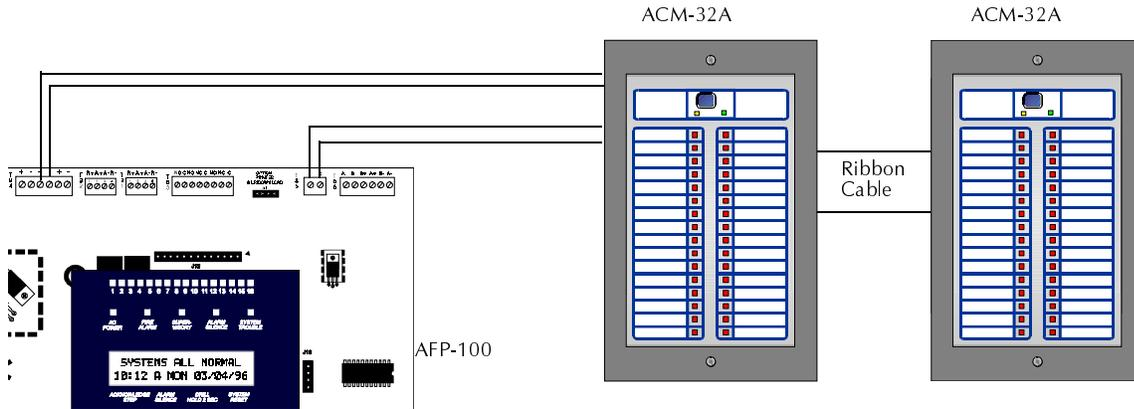
The following configuration provides 16 alarm and trouble LEDs, System Trouble LED, On Line/Power LED, local Silence/Acknowledge, Drill and Reset remote switches and panel sounder. *Only one per system.*
