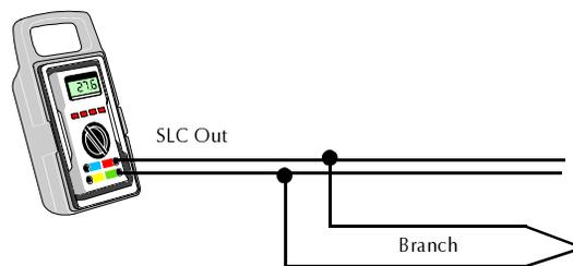
Figure 14 Measuring Resistance on a Two-Wire SLC
