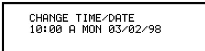
The first digit of the hours is flashing and may be changed with the numeric pad. The right arrow moves to the next digit. The up and down arrows select (A)M or (P)M, day of the week, month, day and year. Pressing the ENTER key stores the time and date and returns to the Level 2 screen.
