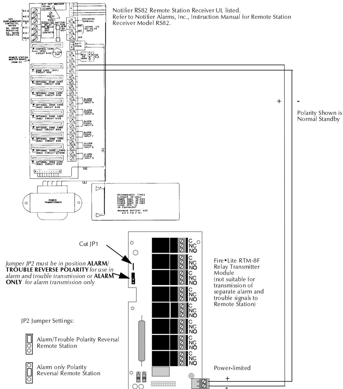
Figure 53 NFPA 72 Remote Station Protective Signaling System
