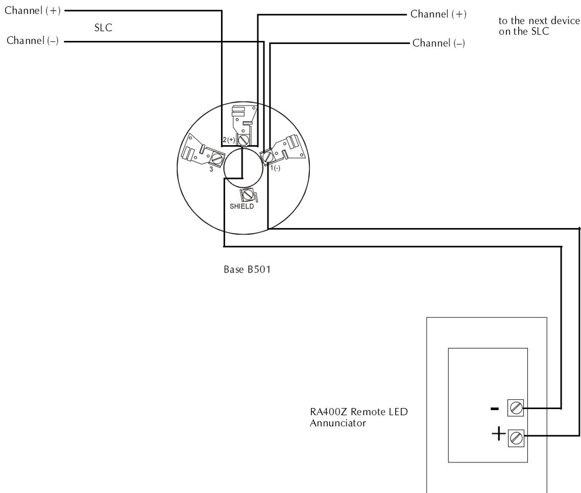
**Figure 36 Wiring Detector with Removable Plug-in Connector**
