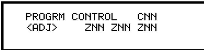
CMX modules default to Zone 00 (general alarm). All Type Code options are silenceable except Relay and Strobes. The selection of CMX module Type Codes may change their function. Select the Type Code from the library list shown in Table 10, using the arrow keys as described in "New Detectors" on page 73.
