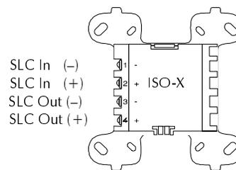
**Note** During a fault condition, the AFP-100 will register a trouble for each device isolated on the SLC branch.
