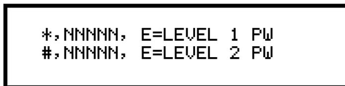
Select the password to change by typing \* or #, then enter the new password. As the new program or status password is entered, it is displayed. When the enter key is pressed, the display reads PRESS ENTER IF OK, NNNNN=NEW PROGRAM PW. After the ENTER key is pressed, the new password is stored in EEPROM memory and the program returns to the program change screen. If BACKSPACE is entered, the password remains unchanged and the program returns to the program change screen.
