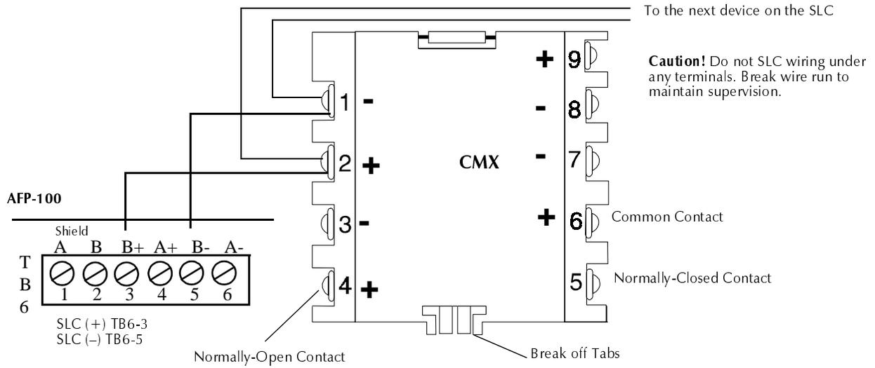
Figure 33 CMX Module - Used as Form-C Relay
