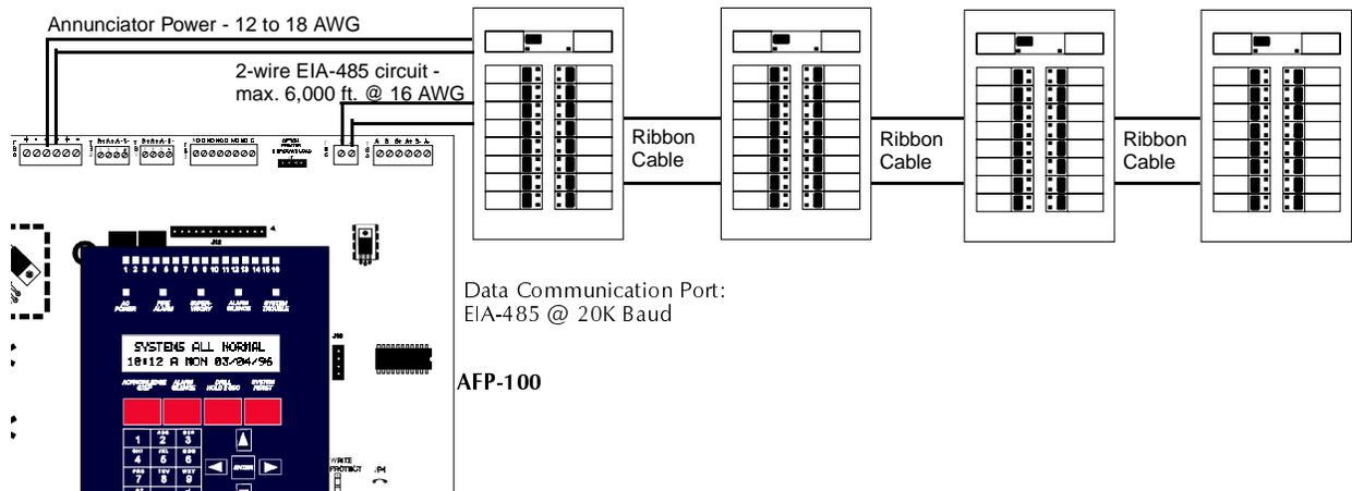
The following configuration provides 56 zones of alarm indication, a System Trouble LED, an On Line/Power LED, local panel sounder and a local Silence/Acknowledge switch.
