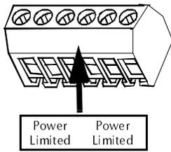
Note: If relays are used as power-limited circuits, paste supplied label to terminal block to indicate use of power-limited wiring.
