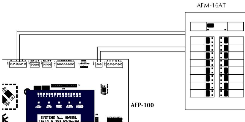
The following configuration provides 32 alarm LEDs, On Line/Power LED, System Trouble LED and local Silence/Acknowledge switch. *Only one per system.*
