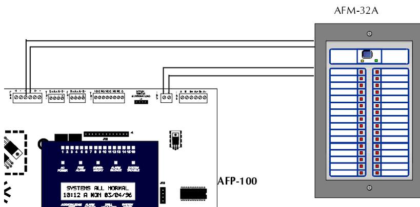
The following configuration allows the annunciation of 56 zones on the first two annunciators. 56 zones are annunciated on the second four annunciators. The same 56 zones are annunciated on the last four annunciators (which duplicate the previous set).
