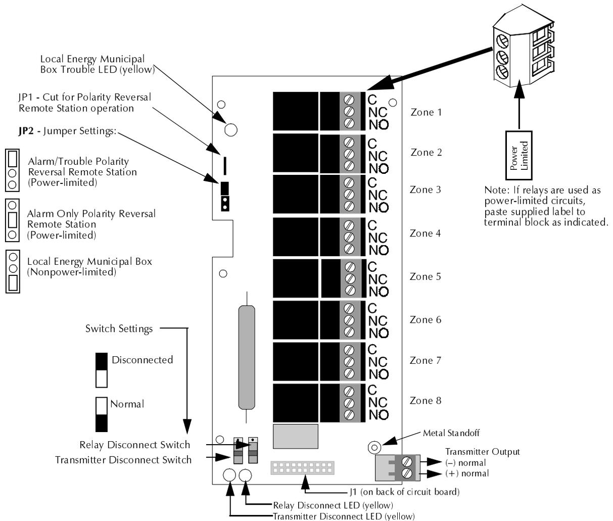
Figure 43 Fire•Lite RTM-8F Relay Transmitter Module Components
