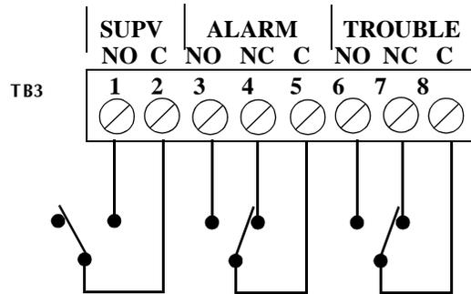
Figure 10 Relay Connections (TB3)
