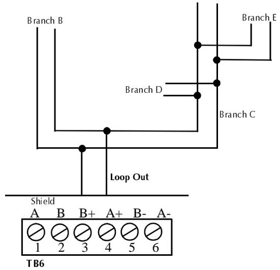
Figure 15 Style 4 T-tapping and Branch Resistance
