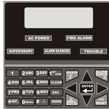
Figure 1.3 Membrane/Display Panel
