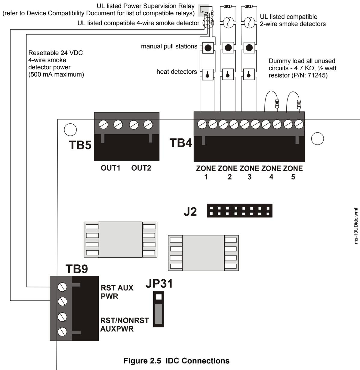
Figure 2.5 IDC Connections
