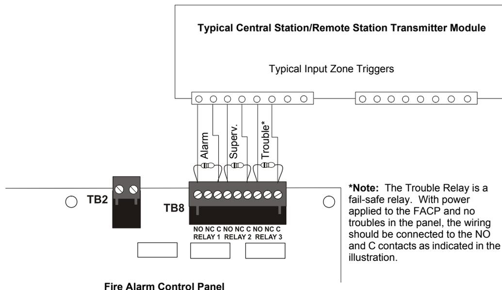
Figure B.5 FACP Dry Contacts Connection to Central Station/Remote Station Transmitter
