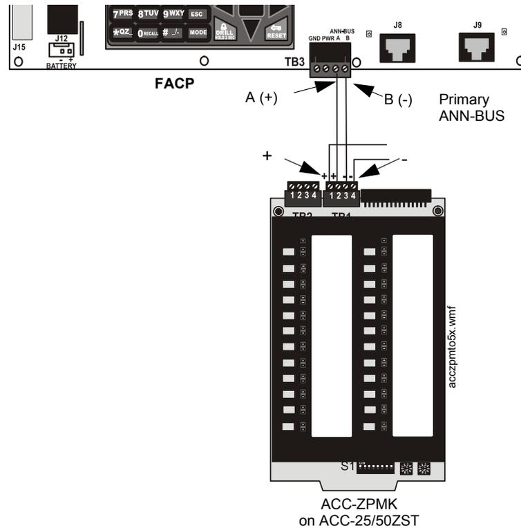
**Figure 2.30 FACP Connection to ACC-25/50ZS/T Audio Panel**
