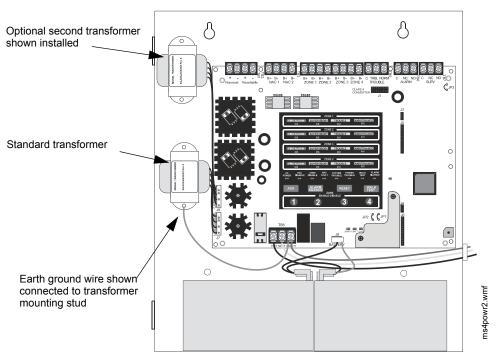
Figure 2.3 Operating Power Connections
