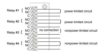
Figure 2.14 4XZMF Zone Relay Module
