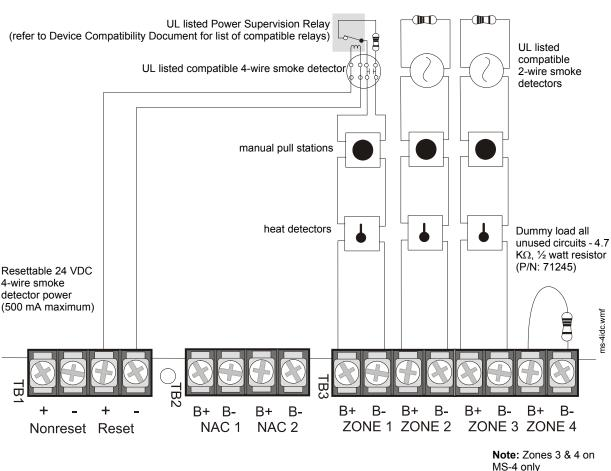
Class B Initiating Device Circuits (supervised and power-limited) 4.7 K\Omega,  $\frac{1}{2}$  watt resistor P/N:71252
