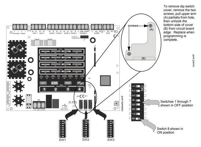
Figure 3.1 Field Programming DIP Switches
