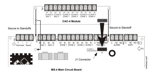
Figure 2.10 CAC-4 Module Installation
