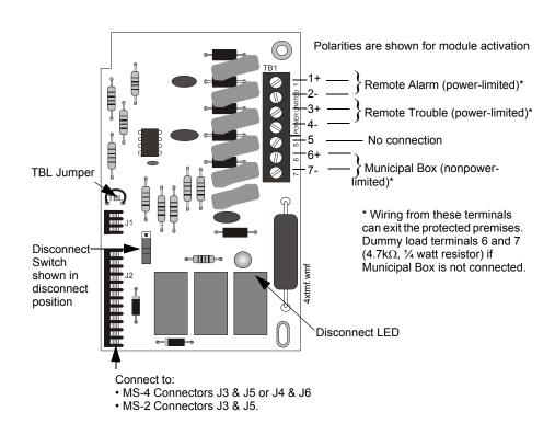
**Note:** 4XTMF Module is not suitable for transmitting reverse polarity supervisory signal.
