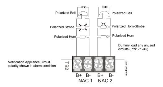
Class B Notification Appliance Circuits (supervised and power-limited)  $4.7 \text{ K}\Omega$ , ½ watt resistor P/N:71252
