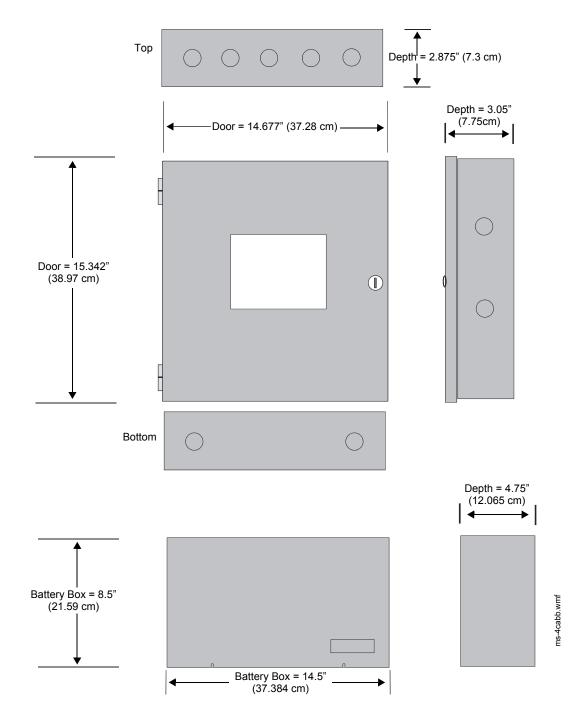
Figure 2.2 Backbox and Battery Box
