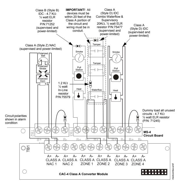
Figure 2.11 Wiring NACs and IDCs for Class A Operation
