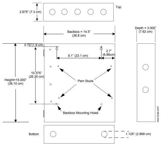
Figure 2.1 Backbox Mounting Dimensions
