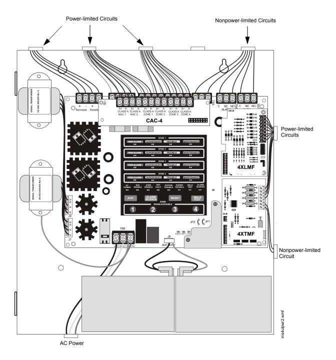
Figure 2.9 Typical UL Power-limited Wiring Requirements
