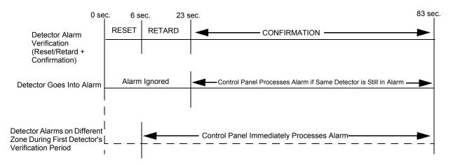
Important! Circuits selected for verification must have only smoke detectors installed
