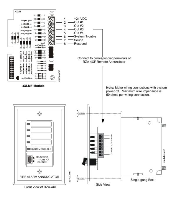
Figure 2.15 4XLMF LED Interface Module
