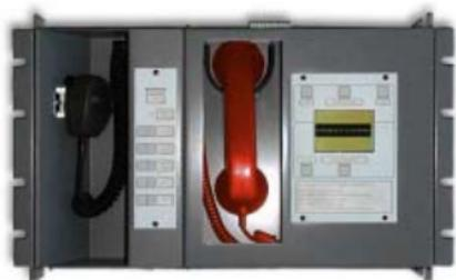
The Audio Source Unit (3-ASU/3-ASUFT) converts analog signals to digital signals. These units support connection of a local microphone, remote microphone, telephone voice line, and auxiliary audio input.
