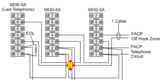
**Note:** Use of "Off Hook" Terminals 3, 4, and 6 are for NFPA 72, 3-state operation (IRC-3 and FCC only).
