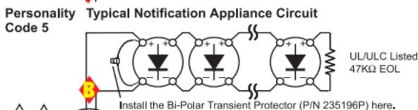
Install the Bi-Polar Transient Protector (P/N 235196P) here.
