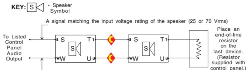
**CAUTION:** Electrical supervision requires wire run to be broken at each device.
