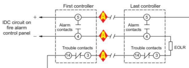
Fire alarm initiating circuit wiring
