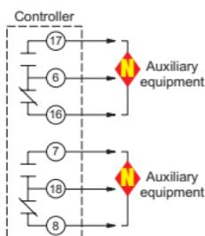
Auxiliary relay wiring
