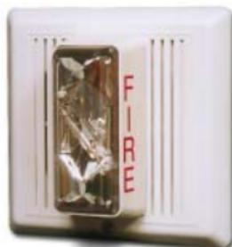
Integrity strobes synchronize to the latest UL 1971 requirements when used with an external control module (G1M or SIGA-CC1S). High efficiency speaker produces a loud 90 dBA at 2 watts. Easy to select for  $\frac{1}{4}$ ,  $\frac{1}{2}$ , 1, or 2 watt operation. Integrity speakers are supplied with a DC Blocking Capacitor for audio circuit supervision.
