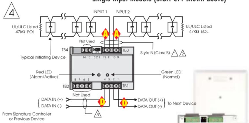
SIGA-UM Class B Dual Input Module (CT-2 wiring shown above)
