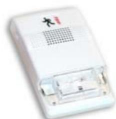
Genesis chimes automatically pulse at 60 strokes per minute, when steady (non-stroked) voltage is applied, or may be field-configured for temporal output. When installed with a GIM Signal Master Module, the chime may also be field-configured for coded operation, which enables the chime output to match the rate that voltage is applied to the circuit. Peak output level is 79 dBA (peak). The chime may be set for low dB output with a jumper cut that reduces sound output by about 5 dB.
