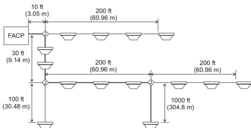
Table C-2 through Table C-5 provide the maximum allowable branch length for any detector, module, SIGA-UM, and wire gauge combination. Using the wire distances specified in the tables ensures that the circuit does not exceed the maximum circuit resistance of the Signature data circuit.
