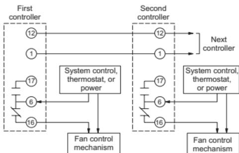
Multiple fan shutdown interconnect wiring
