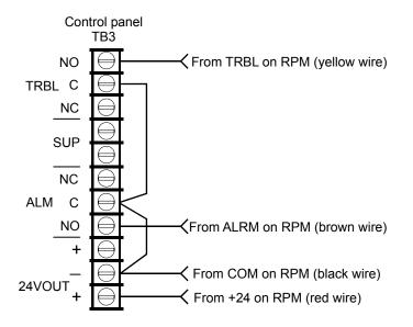
Alarm, supervisory, and trouble transmitted on separate circuits
