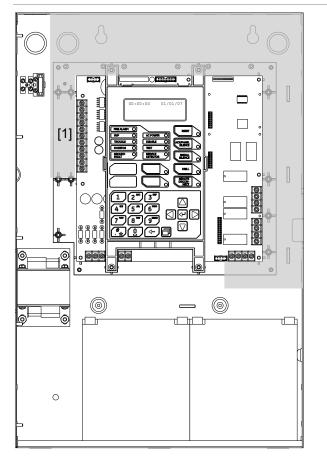
**[1]** Power-limited only when connected to a power-limited source. If connected to a nonpower-limited source, all wiring on terminal block TB3 must be FPL, FPLP, FPLR rated wire or equivalent, in accordance with the NFPA 70 *National Electric Code* and routed separate from all power-limited wiring.
