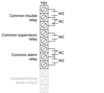
Note: Diagram is shown with the panel in a normal state.
