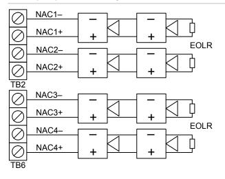
250/500 point panel Class A wiring
