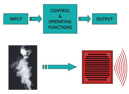
Figure 2-1. Three Fire Alarm System Parts
