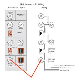
The first device in the Maintenance Building wiring diagram is the Maintenance Office Smoke
