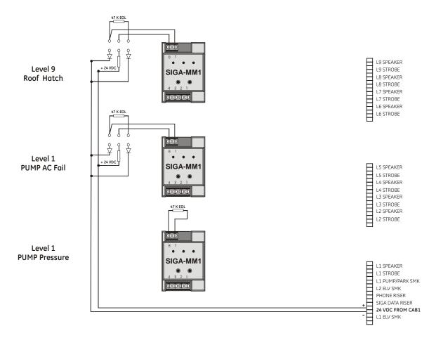
MacNeill Plaza Main Building Monitor Module Simulation Wiring
