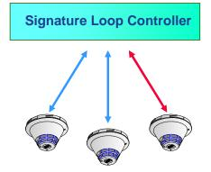
The loop controller communicates with each device until the device in a new start condition with the highest serial number is determined
