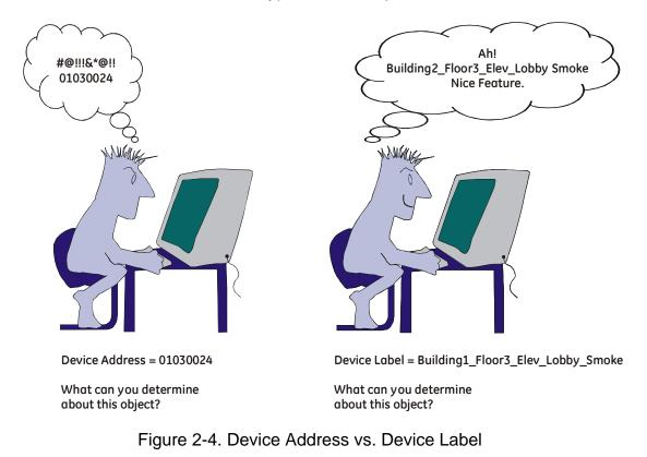
In the example above, both the device address and the device label identify the same smoke detector in the elevator lobby, located on the third floor of a multi-floor building, in the second building of a multi-building complex.
