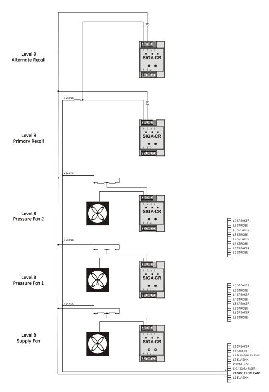
MacNeill Plaza Main Building Control Relay Simulation Wiring
