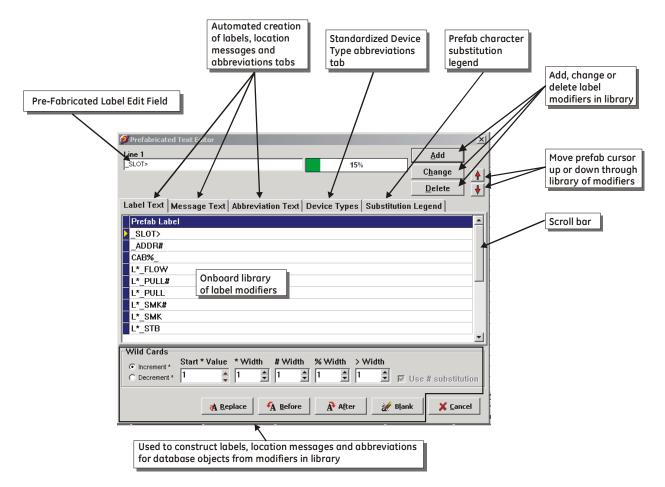
Figure 2-6. Prefabricated Text Editor
