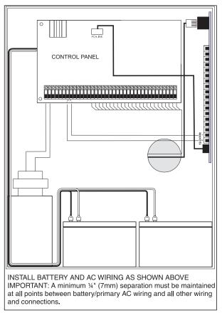
T-Link board must be mounted on the side of the cabinet. Refer to the mounting instructions in the associated Installation Manual.
