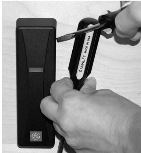
FIGURE 2: Removing the reader cover
