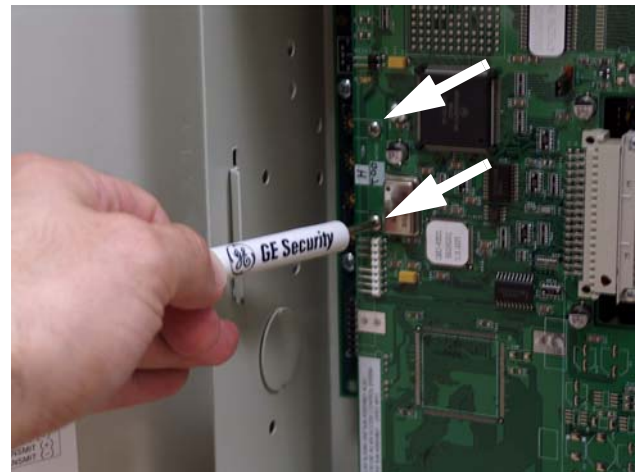
Figure 1. Removing the screws holding in the CPU board
