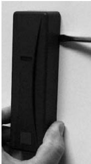
Figure 4. Removing the Cover
