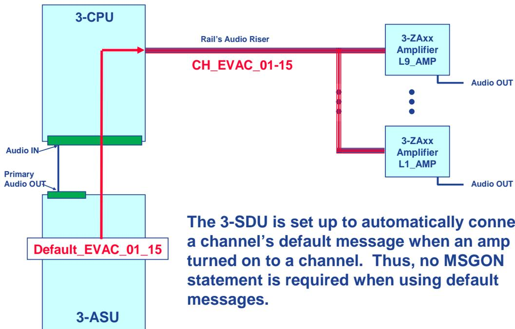
The 3-SDU is set up to automatically connect a channel's default message when an amp is turned on to a channel. Thus, no **MSGON** statement is required when using default messages.
