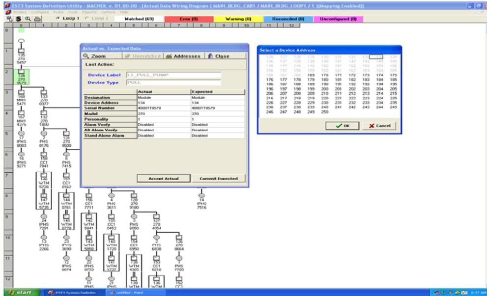
1. The Select a Device Address dialog box appears displaying the address assigned
