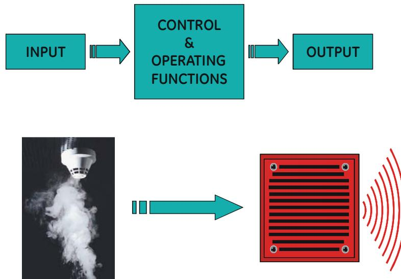
Figure 2-1. Three Fire Alarm System Parts
